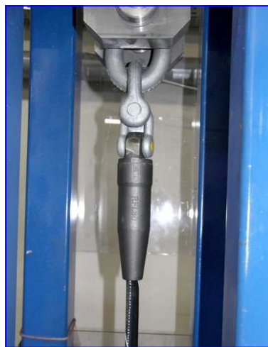
Cable Ø27 with connector RFI 30 Breaking of the cable at 23T
