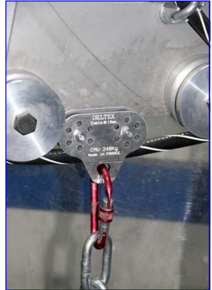
Breaking test of the pulley model P61
