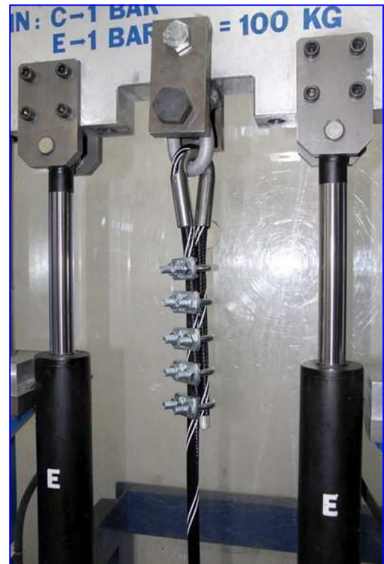
Cable Ø19 mm with thimble and 5 cable clamps Breaking at 7T
