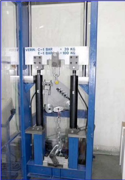
Breaking test of the pulley model P68
