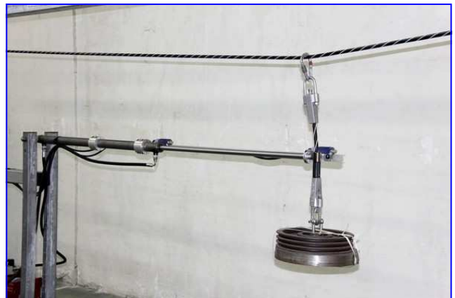
The screw jack pushes a weight of 65 Kg hanged to a carabiner, 420 passing per hour. After 36 hours of testing, the usury is of about 1/10 th of a mm.
