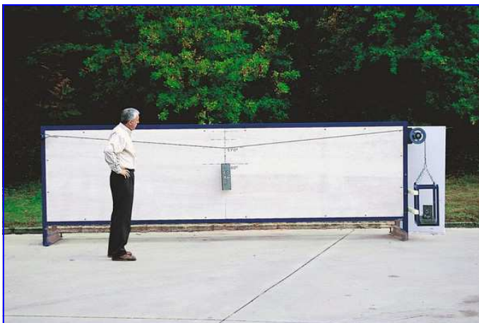
The 10 kg weight lifts a counterweight of 58 kg and finds equilibrium at 170° .
