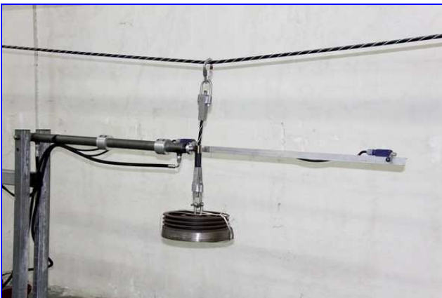
Wear and tear test by rubbing a carabiner on a belay wire's cable Ø 15 square wire
