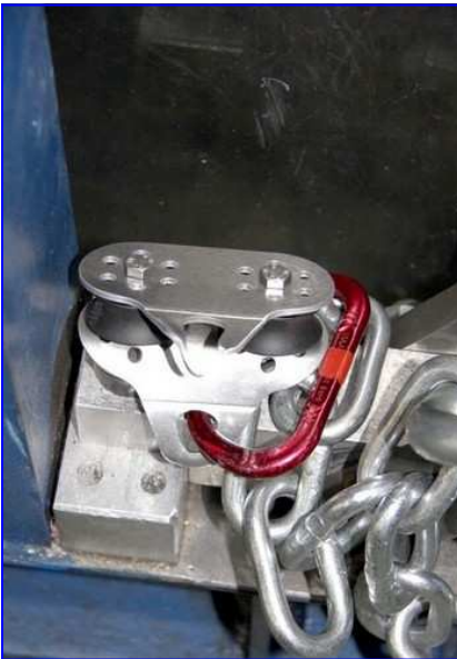
Breaking of the bottom of the pulley at 1980 KgF
