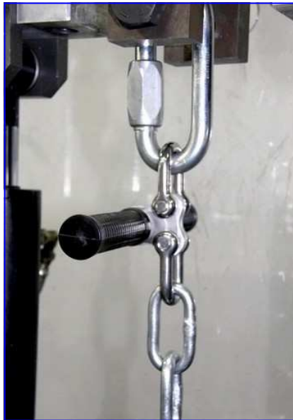
Breaking test of the handles
