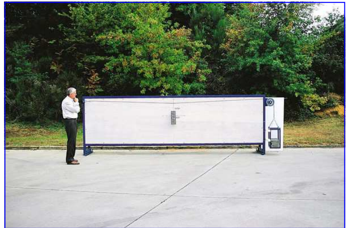
In the photo above, the 10 kg weight lifts a weight of 127 kg and brings the cable to 175° .
